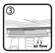
Pull filter towards front of vehicle and remove, Fit new Ryco RCA135C. close and lock housing door.
