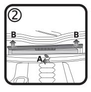
Unlock at "A" then swing door open by holding at "B" and lifting.
